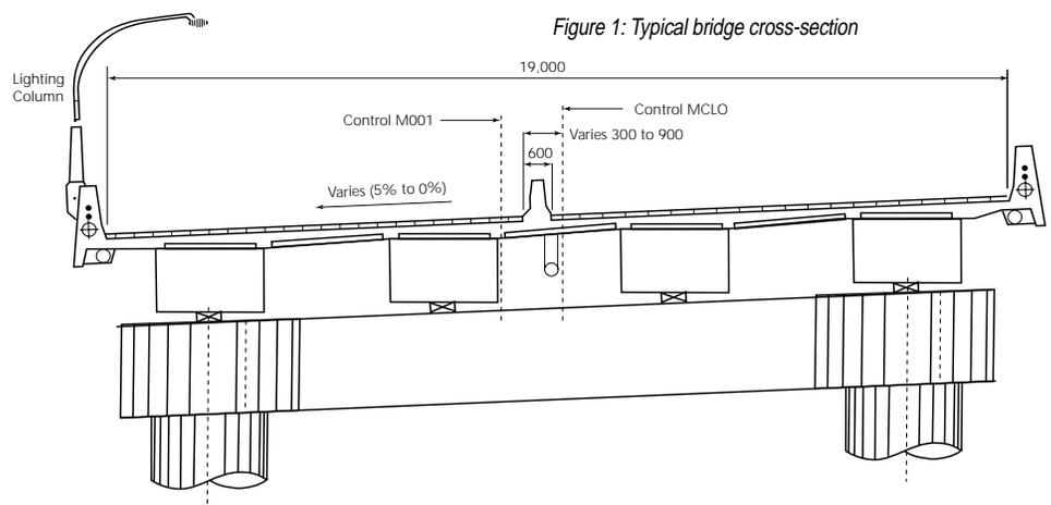
Figure 1: Typical bridge cross-section
