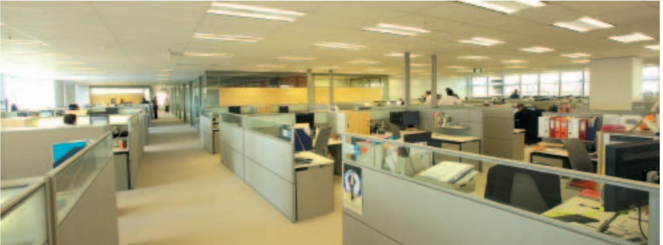
The column-free floor plate of the base building allowed the fit out design by Woods Bagot to incorporate a continuous subdivision module that allows all work point types to be interchangeable across the space and throughout the tenancy.
